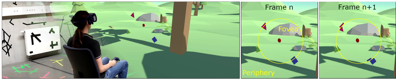
Figure 1: In our user study, participants tracked objects in virtual reality under different frame rates and scene environments. Frame n shows the fully rendered environment, in frame n + 1 , the periphery is unchanged and only the foveal region is rendered freshly. Forest Asset courtesy of Oleh Lila, used with permission.
