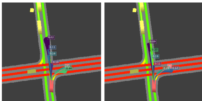
Fig. 3: Visualization of the predicted trajectories with estimated position uncertainties. The circles are centered on the predicted positions and the radius corresponds to two times the predicted standard deviation.
