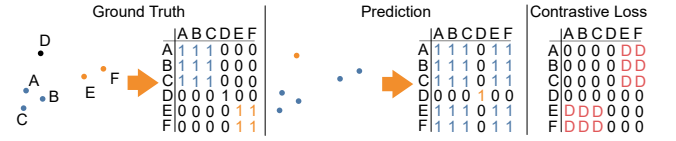
Figure 3: Visualization of the encoding of ground truth and predicted clusters, along with the corresponding contrastive loss. Scattered data with color coded clustering (left), and corresponding similarity matrix \mathbb{S} , see Equation (1) (right).
