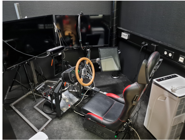
Fig. 2. The room for the thermal comfort recordings. The employed air conditioning unit can be seen to the right.
