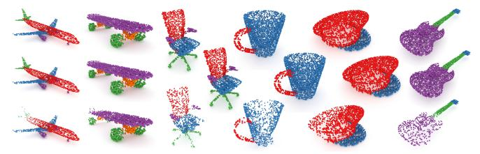
Fig. 9. Comparison of our segmentation result for uniform (second row) and non-uniform samplings (third row) to the ground truth (first row). Non-uniform sampling use the Gradient (first and second columns), LAMBERT (third and fourth columns), and SPLIT (fifth and sixth columns) protocols.
