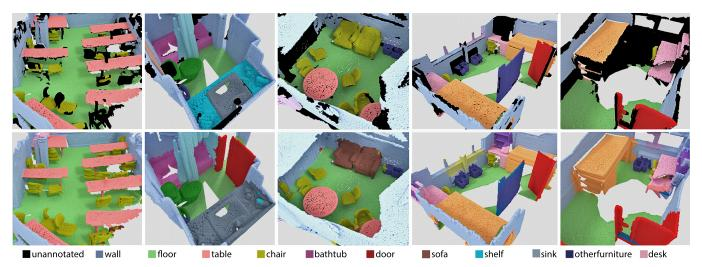
Fig. 10. Semantic segmentation results of our approach (bottom row) on ScanNet [Dai et al. 2017] compared with ground truth (top row).
