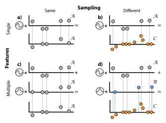
Fig. 5. Monte Carlo convolution for the same / different sampling (horizontal) and a single / multiple feature channels (vertical). Samples are denoted as dots, whereby lines indicate if samplings match. Colors indicate the samplings  $\mathcal{A}$ ,  $\mathcal{B}$  and  $\mathcal{C}$ .
